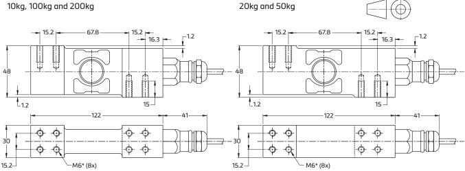
Mounting bolts M6 8.8; torque 10 Nm. Torque value assumes oiled threads. \* Unified thread 1/4-20 UNC is available.
